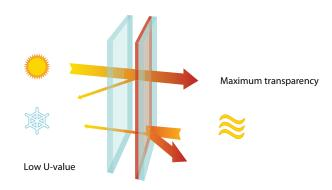
GUARDIAN ClimaGuard<sup>®</sup> A 1.0 promotes well-being: The increased insulation results in a higher internal glass surface temperature, reducing the occurrence of condensation and uncomfortable cold spots and down-draughts close to the window.
